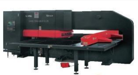
Multi station CNC punching machine
