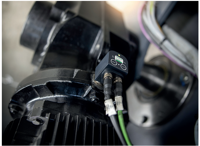
Condition monitoring solution Logistics center: SmartCheck monitors rack feeder motors
